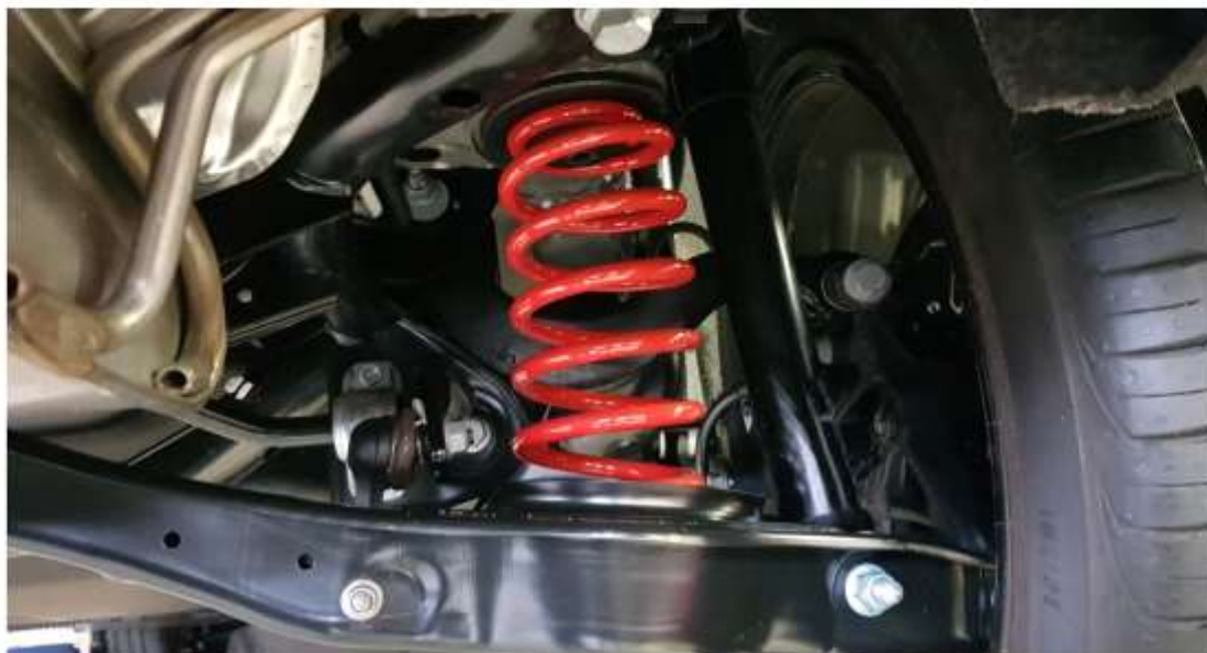
Lowering spring mounted on car - rear suspension
